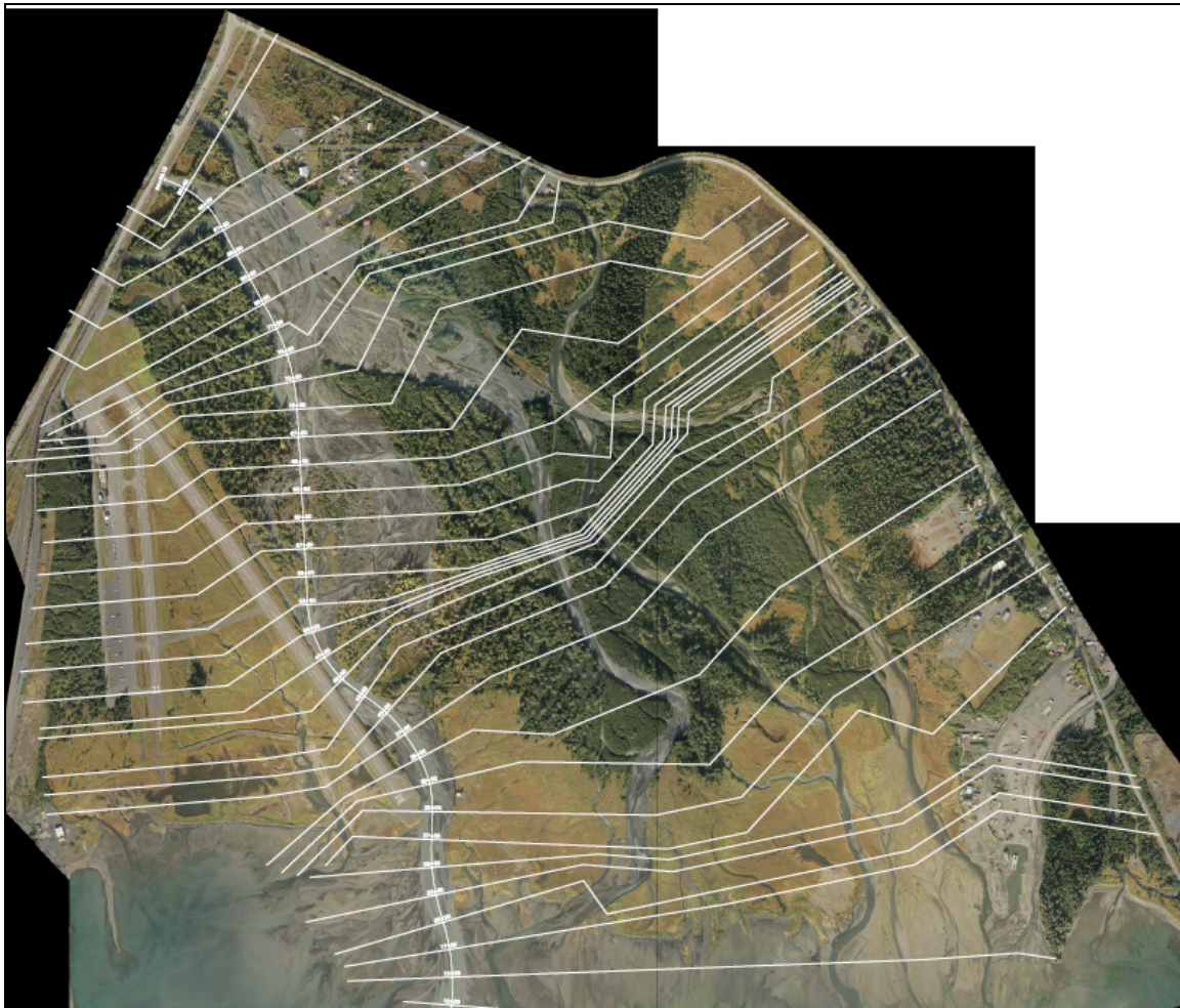
Figure 39: Aerial Photograph of Resurrection River Delta showing the location of hydraulic cross-sections.
