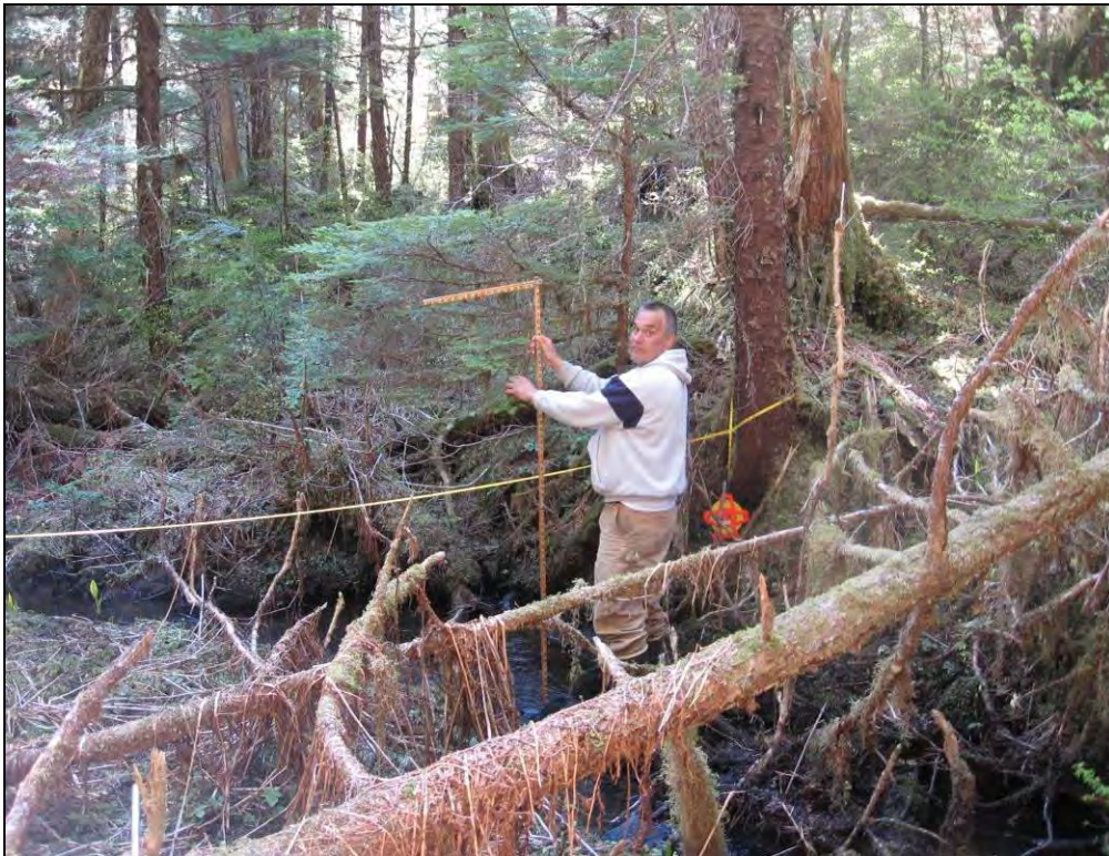
Photo 11. Stream 1. Photo was taken approximately 50 feet downstream of Access Alt. 2 road crossing. FAA's consultant team member is measuring the stream cross-section.
