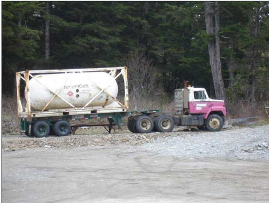
Figure 4: 20-foot mod for transporting propane.
