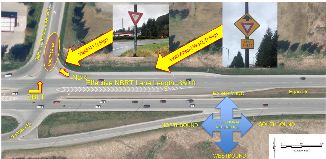
Figure 1- Existing Geometric Conditions
