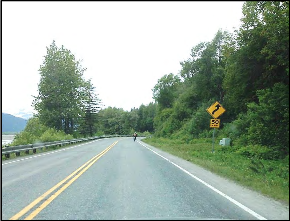
Photograph 2.0-1: Bicyclist on Highway with Narrow Shoulders (Photo courtesy of Bob Trousil, P.E., DOT&PF, May 2014)
