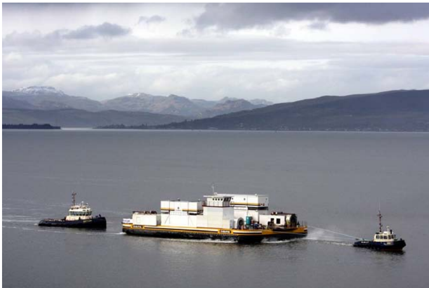
Figure 4-2. Siberian Hoverbarge with 200 ton payload by Hovertrans
