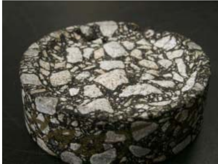
Figure 6.8. A cylindrical asphalt mixture sample after Prall testing.
