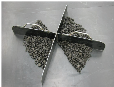
Equal portion from the diagonally opposite quarter
