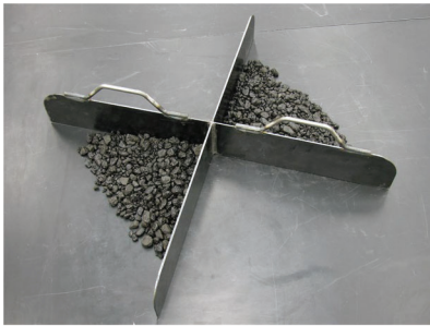
Diagonally opposite quarters removed
