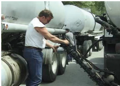
Sampling from the spray bar
