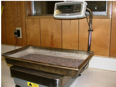
Determining Initial Dry Mass
