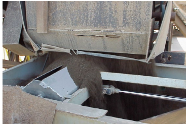
Automatic Sampling Device in Stream
