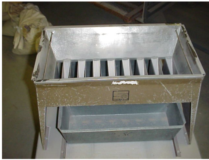
Mechanical (riffle) splitter
